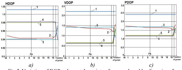
*Fig.2.* Variation of DOP values at the points of approach and landing aircraft trajectory
